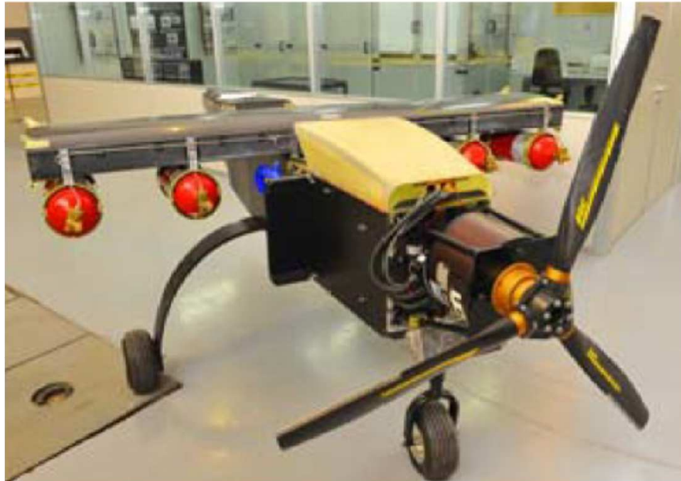
INTA electrical propulsion system for small aircraft – electrical configuration
