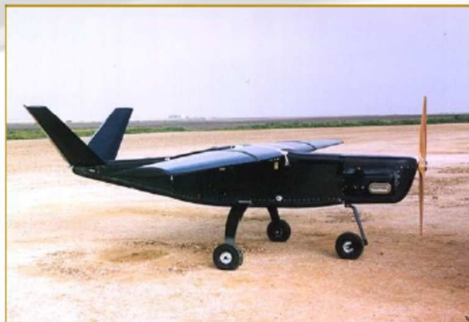
INTA electrical propulsion system for small aircraft – electrical configuration
